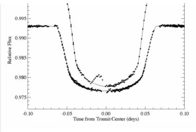
Fig. 1: Transit light curves of two transiting exoplanets, TrES-1 (top) and HD 209458 (bottom, offset by -0.007 for clarity). Since TrES-1 has a shorter orbital period and smaller size, the transit duration as well as the duration of ingress and egress are shorter. The hump in the TrES-1 data is likely due to the planet occulting one or more star spots on the surface of the star.
