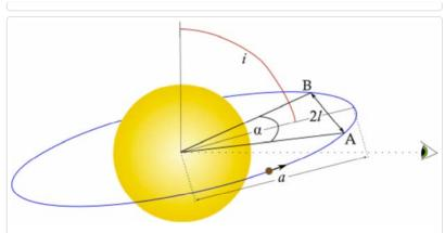
Fig. 4: During a transit the planet moves from point A to B on an orbit with inclination i. For an observer far away, the planet coveres the distance 2l. Assuming a circular orbit, the distance around a full orbit is 2\*pi a where the planet moves along an arclength alpha a between points A and B. From the triangle formed between A, B and the center of the star, sin(alpha / 2) = l/a.
