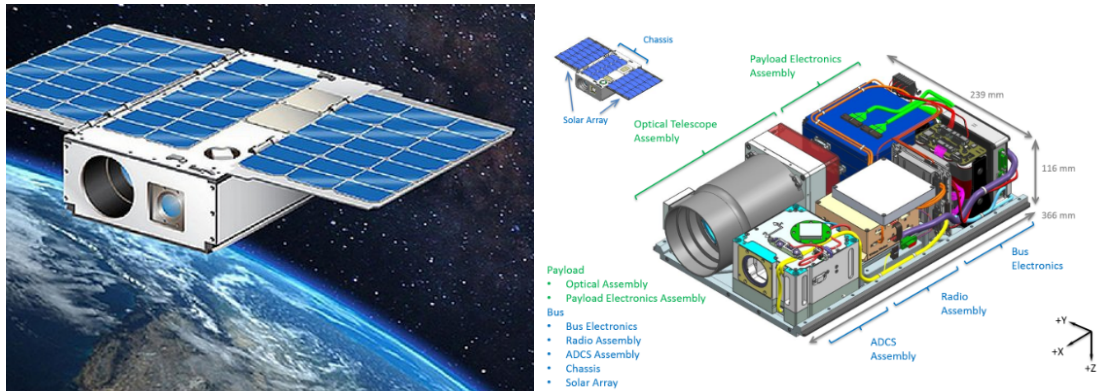
Figure 5. CubeSat with solar panels deployed. (Credit Knapp 2019)
