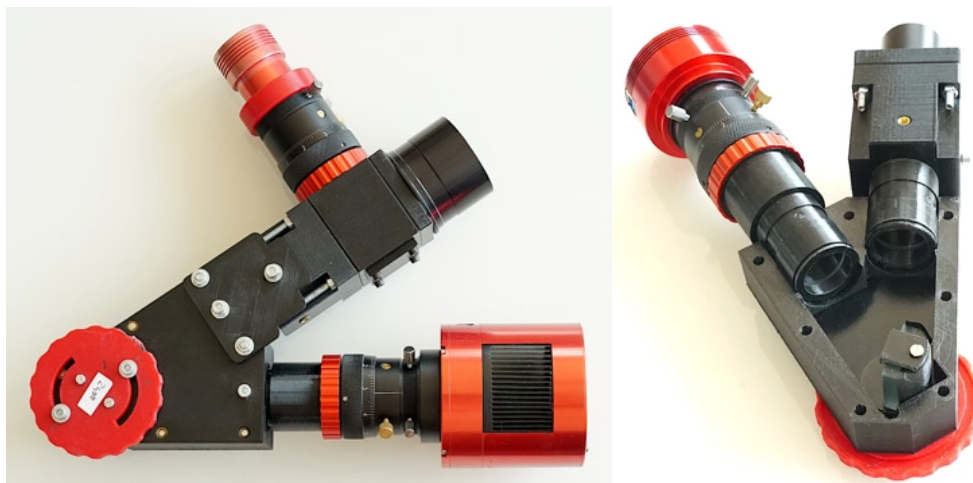
Figure 4. A completed StarEx equipped with the same set of cameras as shown above with the LowSpec. The cut-away on the right shows the simplicity of the interior. The cut-away shows the Solex version which does not have a guide module.
