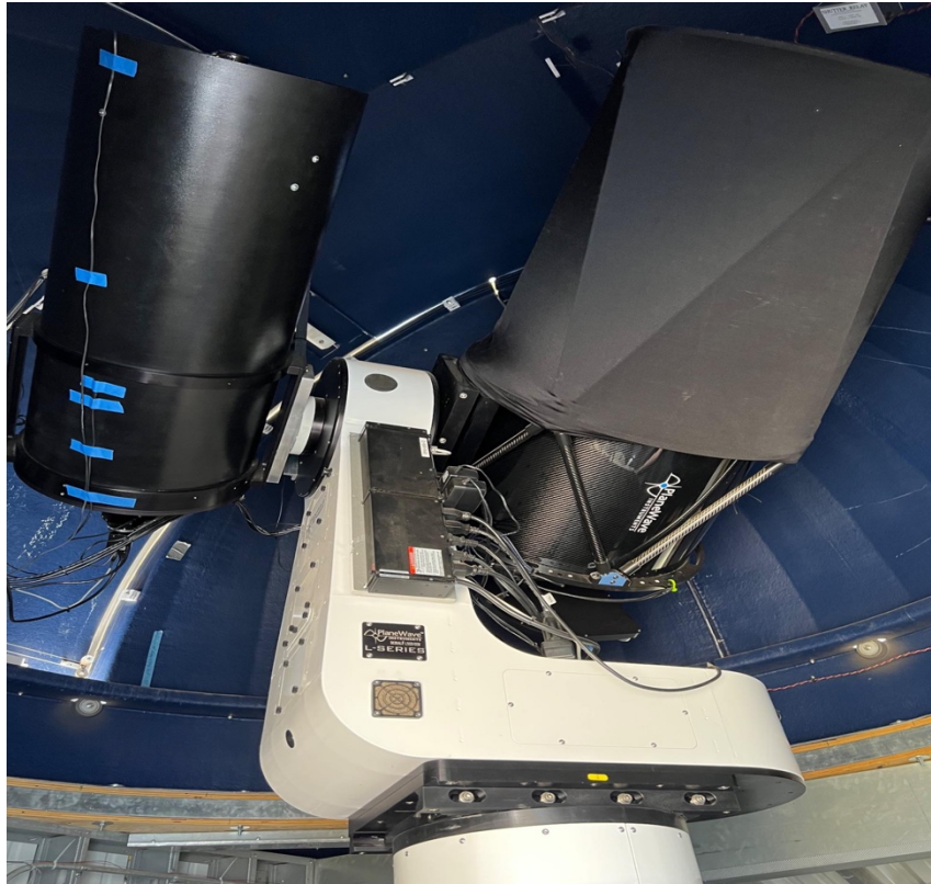
Figure 1. Photometry data presented in this work were collected using the Lowell Observatory's Titan Monitor (TiMo), a robotic 0.5 m PlaneWave CDK20. TiMo is equipped with a CCD-based photometer with a Sloan u'g'r'i'z' filter set, as well as 13 narrowband (10nm) filters from 430 to 940nm.
