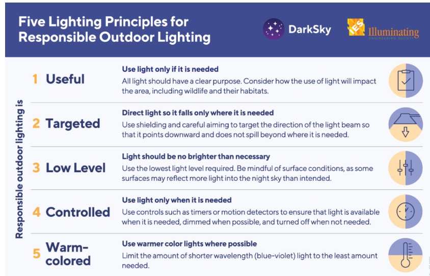
Figure 1. The five principles for responsible outdoor lighting, as articulated by DarkSky International and the Illuminating Engineering Society.
