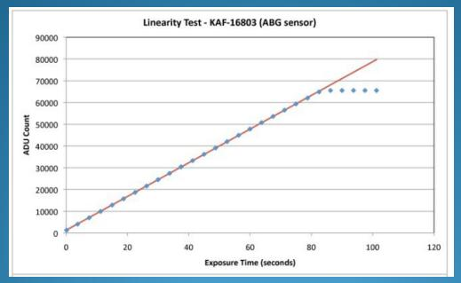
The linearity and saturation point of CMOS chips depends on the readout mode and the gain and offset settings. You have to determine this yourself.
