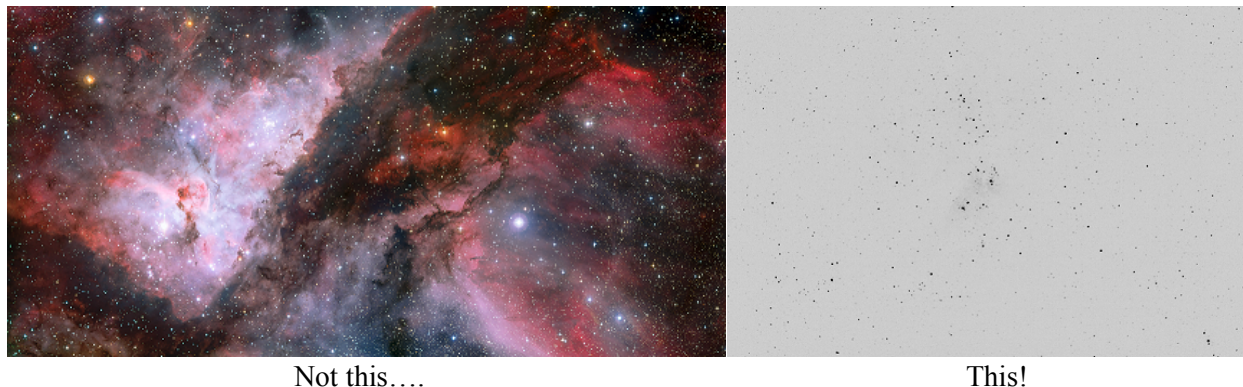
Figure 1.3. What you should, and should not, expect to see in DSLR photometry. Left panel: spectacular image of eta Carinae nebula central region (ESO 2.2m telescope at La Silla Observatory in Chile). Right panel: wider field of view image of same region, 20 sec exposure with 80 mm f6 refractor and Canon 600D DSLR, green channel image. (Mark Blackford)
